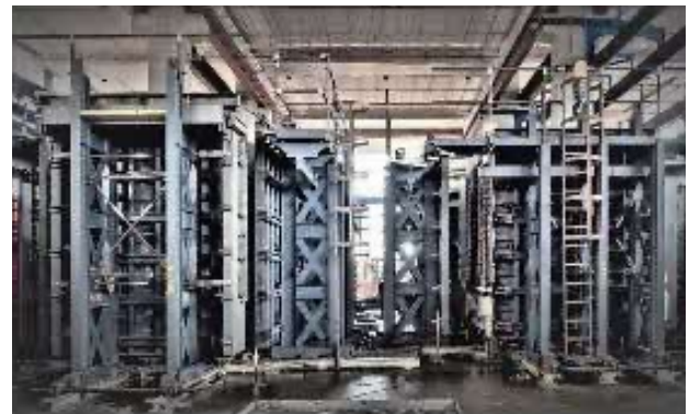
Figure 9: 3D flexible mould.
