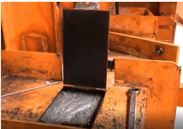
Figure 13: “Concreting inspection” point for 3D PPVC casting on external mould.
