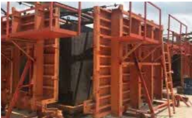
Figure 8: Conventional 3D mould.
